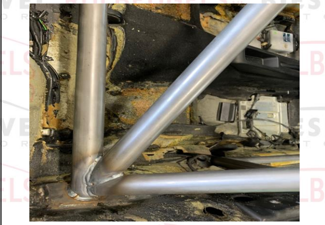
PHOTO 12 SHOULDER HARNESS ATTACHMENT - DRIVER
