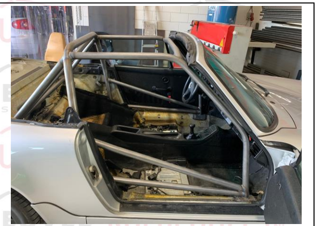
PHOTO 11 ANTI-INTRUSION DOORBAR - CO-DRIVER
