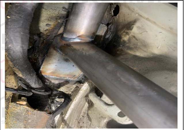
PHOTO 4 MAIN ROLLBAR TO FLOOR ATTACHMENT
