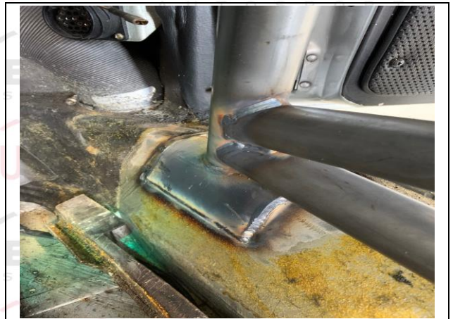
PHOTO 6 FRONT ROLLBAR TO FLOOR ATTACHMENT
